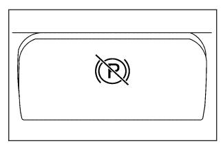
To release the parking brake, hold the regular brake pedal down. Pull the bottom edge of the lever, located above the parking brake pedal, with the parking brake symbol, directly rearward to release the parking brake.
